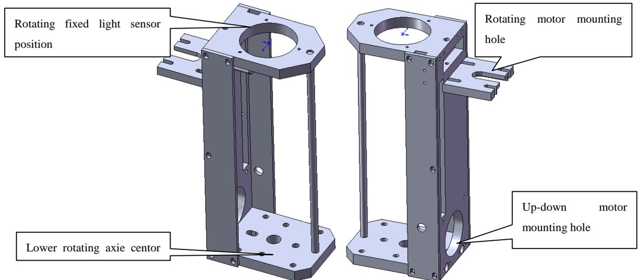
figure 4-2 Probe body and rotating body
