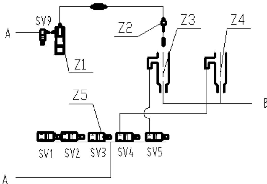
Explanation: Z1—syringe pump unit; Z2—sample reagent probe; Z3—probe rinsing bath; Z4—stirring rod rinsing bath; Z5—five-valve plate unit; A—water tank; B—waste outlet
