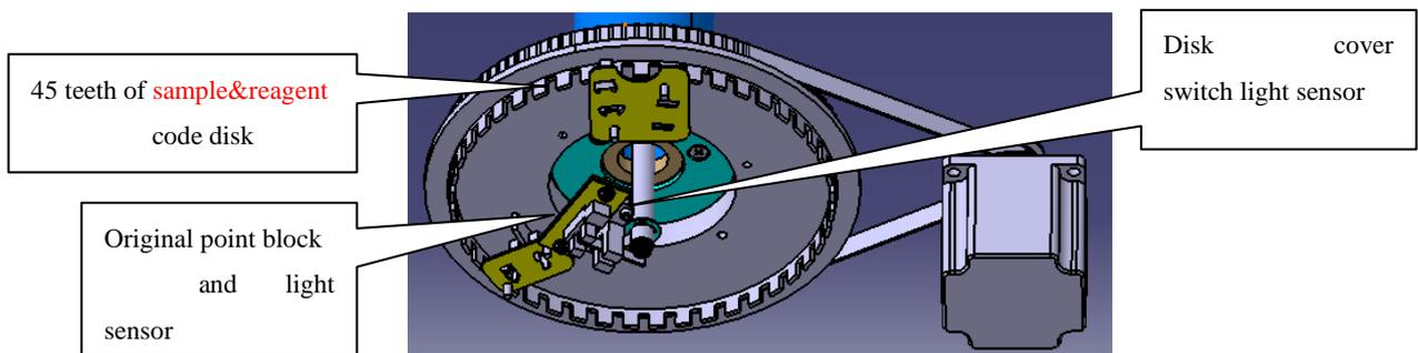
4-7 sample & reagent disk transmission code disk configuration
