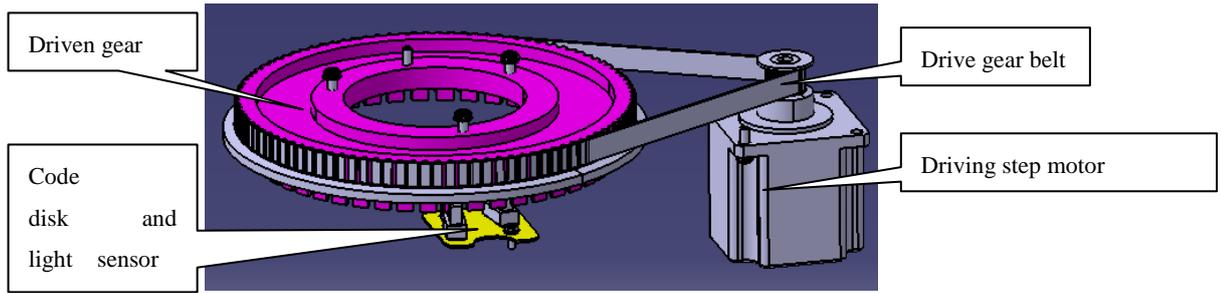
4-5 sample & reagent disk motor driver configuration
