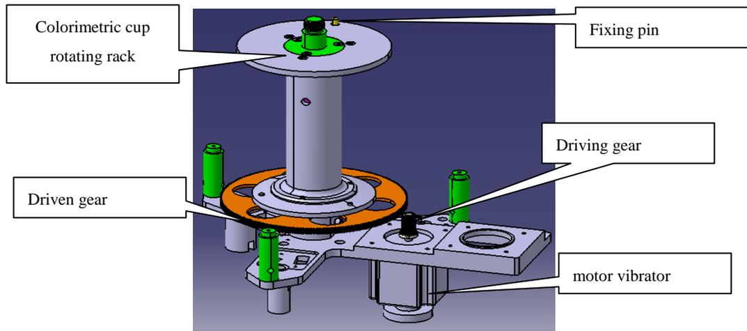
4-10 reaction disk assembly configuration
