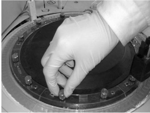
Put on protective gloves to remove fixing screws.
