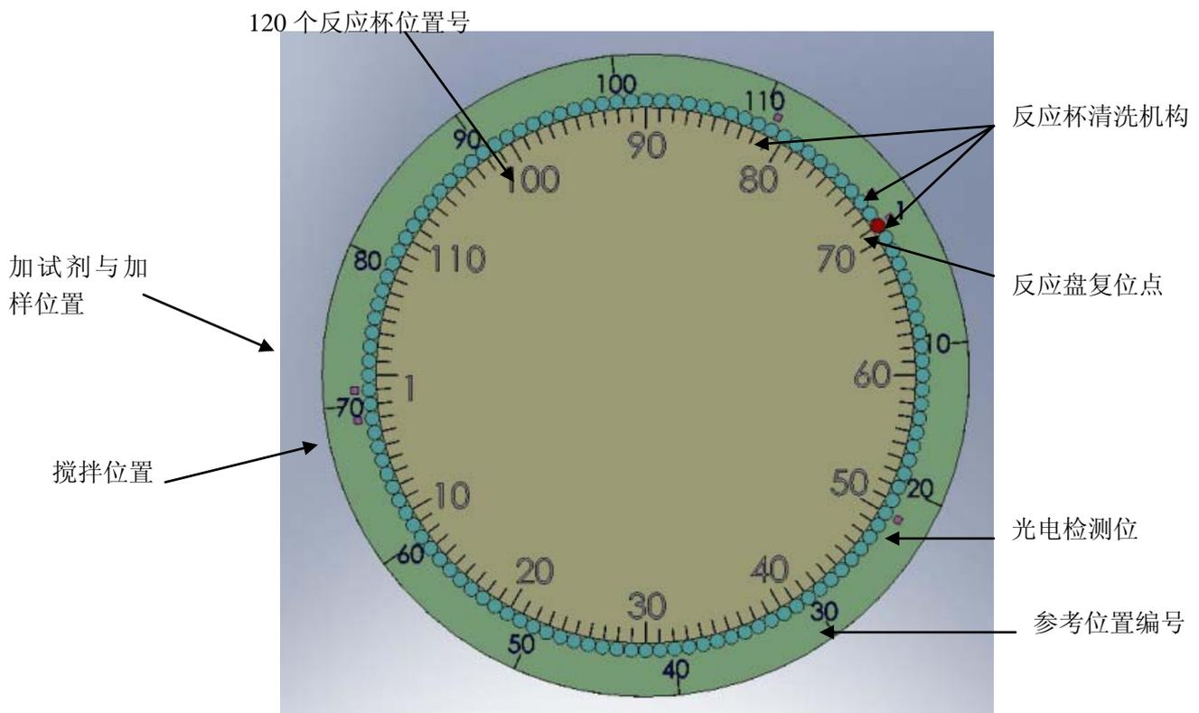
figure 3-2 Position of reaction disk and probe
