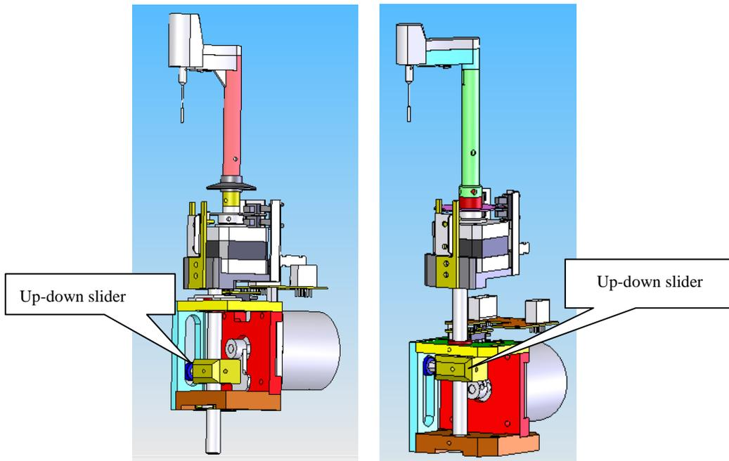
4—19 stirring mechanism up and down positions
