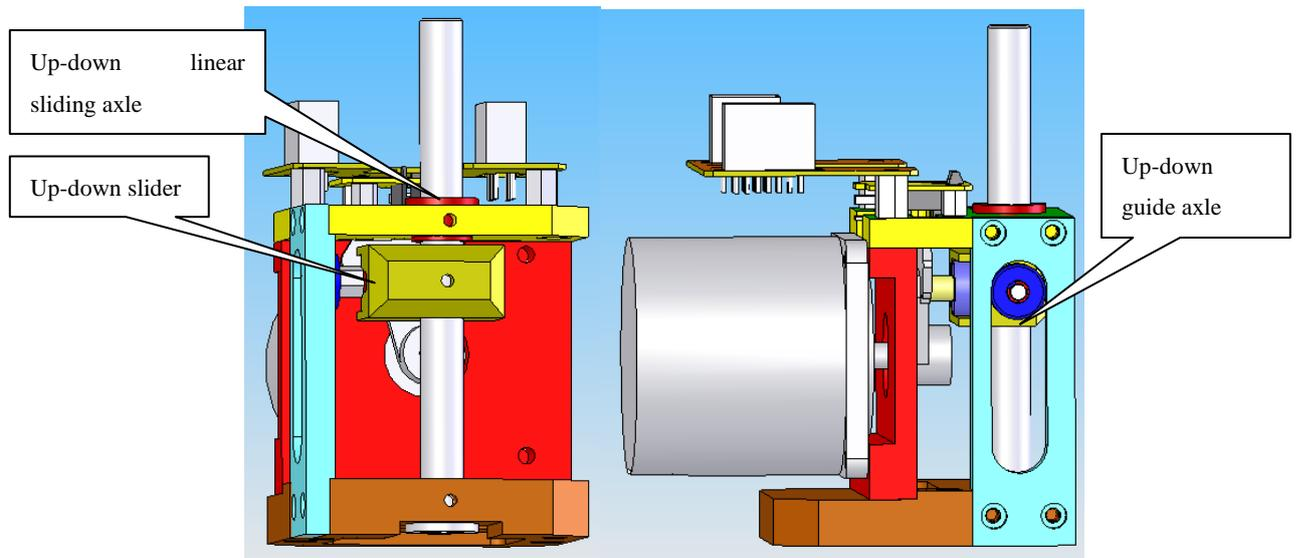
4-18 stirring up-down slider drive configuration
