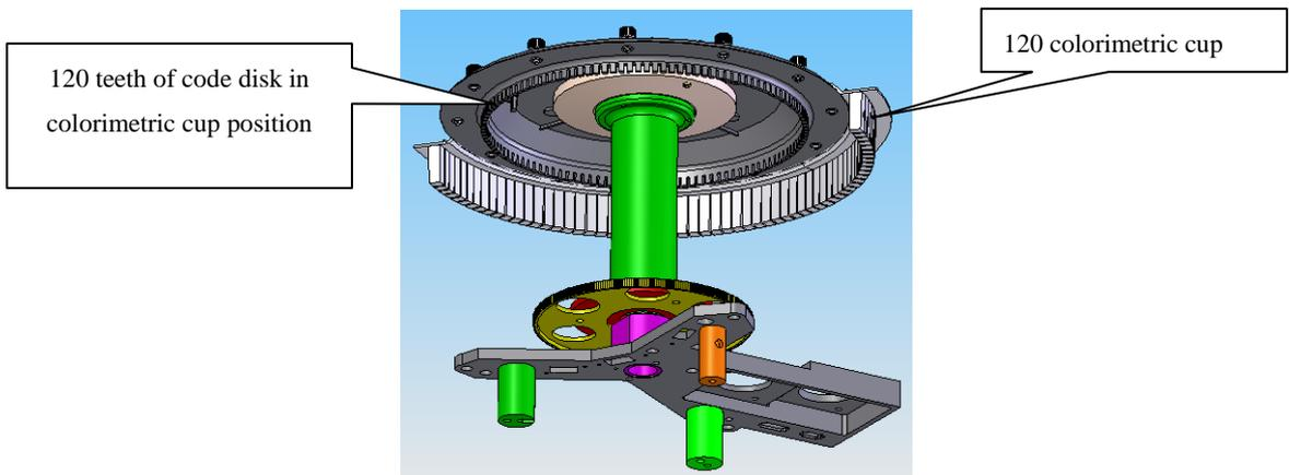
4-11 reaction cup installation disk assembly configuration (1)
