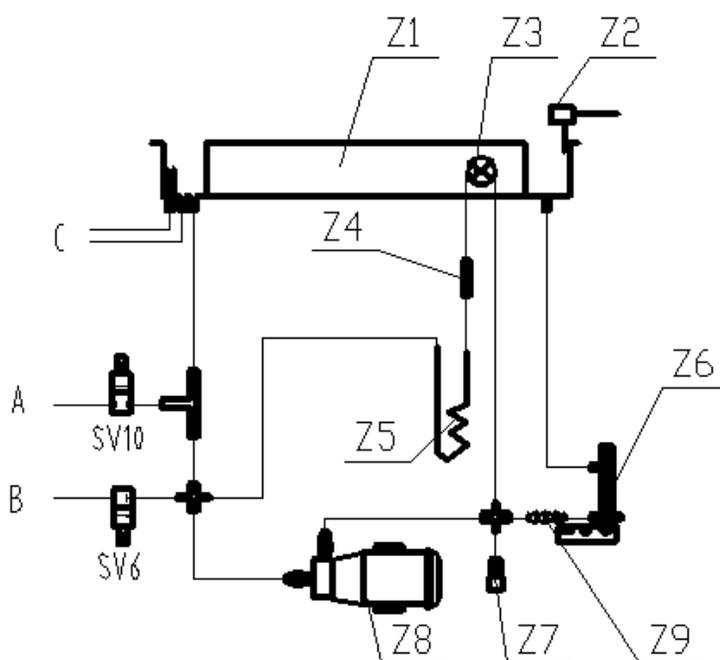
Explanation: Z1—incubation bath; Z2—liquid level detector; Z3—halogen lamp; Z4—flow controller; Z5—lamp cooler; Z6—constant temperature unit; Z7—block; Z8—magnetic pump; Z9—flow controller; A—incubation bath water outlet; B—incubation bath water inlet; C—overflow outlet
