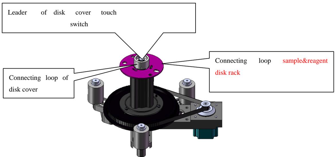
4-6 Sample/reagent disk assembly configuration
