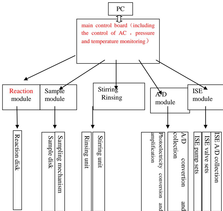
Figure 6-1 Hardware main frame
