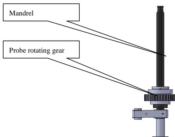
Rotating probe drive ratio is 12:34, using 0.9° stepper motor and 8 segment controller. Control accuracy can achieve 0.0398°.
