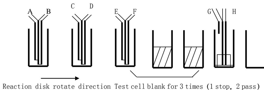
figure 3-3 Reaction cuvette rinsing probe position
