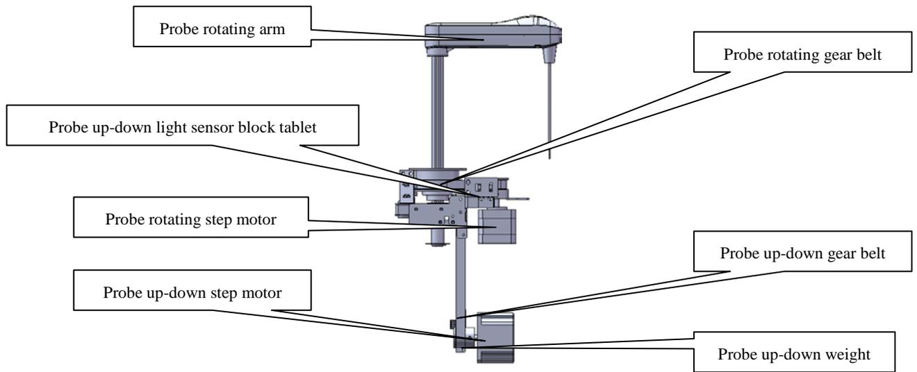
Figure 4-1 probe components configuration
