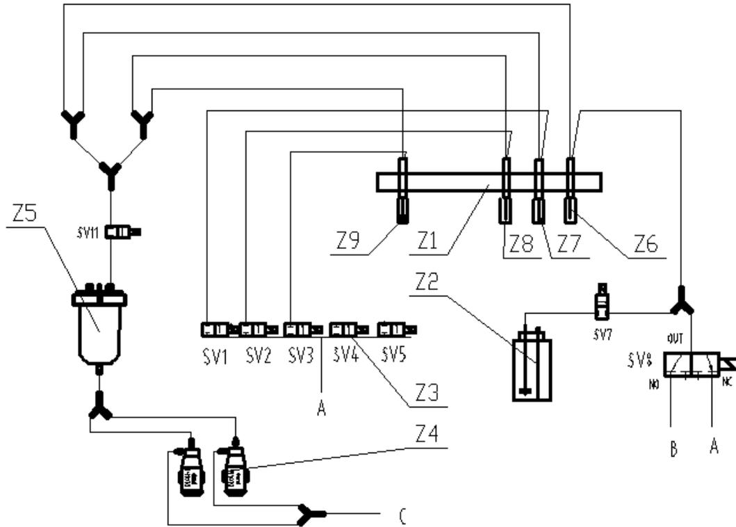
Explanation: Z1—cuvette rinsing unit; Z2—detergent component; Z3—five-valve plate unit; Z4—vacuum pump unit; Z5—liquid collection vacuum tank unit; Z6—nozzle1; Z7—nozzle 2; Z8—nozzle 3; Z9—nozzle 4; A—water tank; B—liquid collection vacuum tank; C—high concentrate waste outlet
