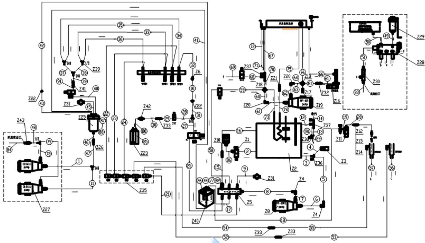
five-valve plate assembly, used for cuvette rinsing, stirring rinsing and external wall rinsing of the probe; second pass through the degassing device for the internal wall rinsing of the probe; third pass with the detergent used for the first probe rinsing of rinsing unit; fourth pass for the incubation bath; fifth pass access to pressure sensor for detecting the tank pressure; sixth pass for regulating the water tank pressure.
