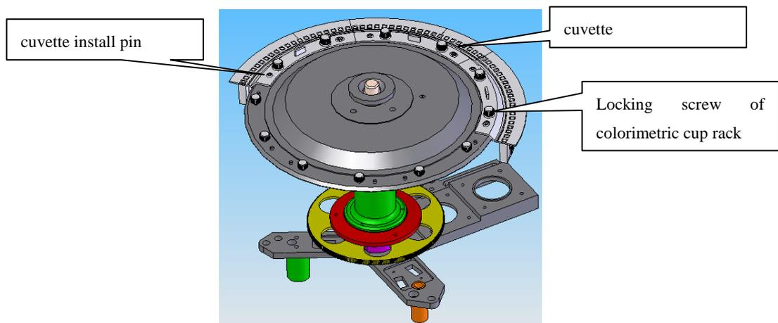
4-12 reaction cup installation disk assembly configuration (2)
